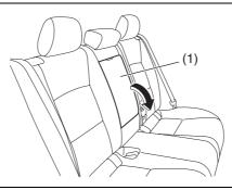
The armrest (1) is stowed in the center of the seatback. Tilt it down forward to use.
